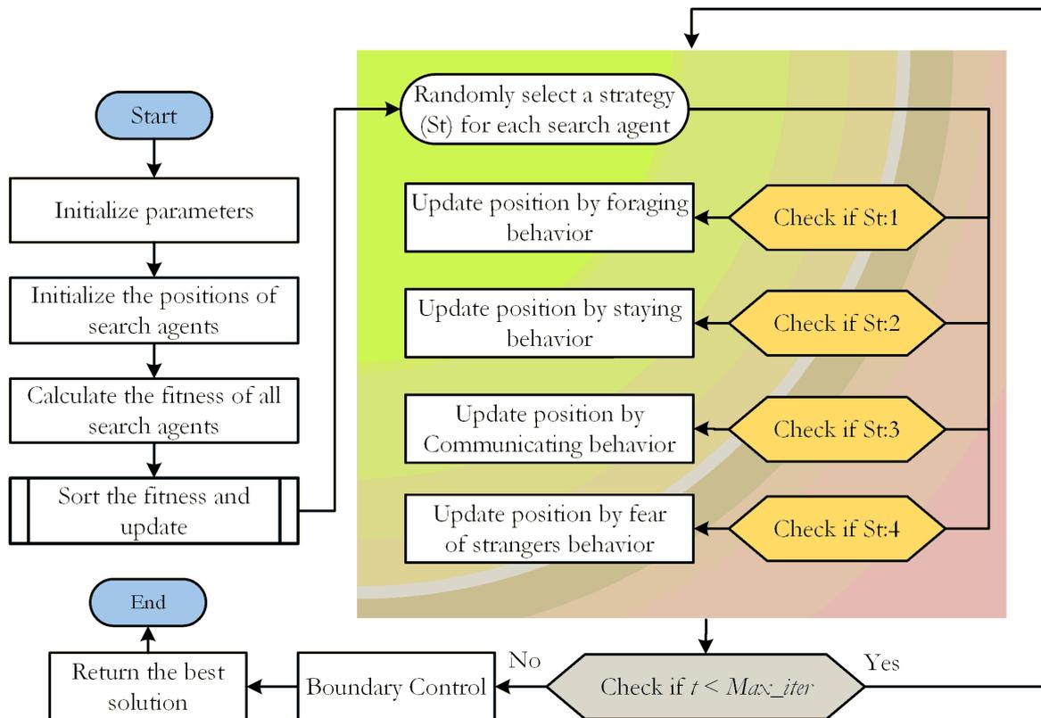
**Fig. 6.** Flowchart of PO algorithm
